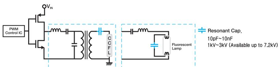
Fig. 3. Typical electronic ballast circuit and MLCC application
