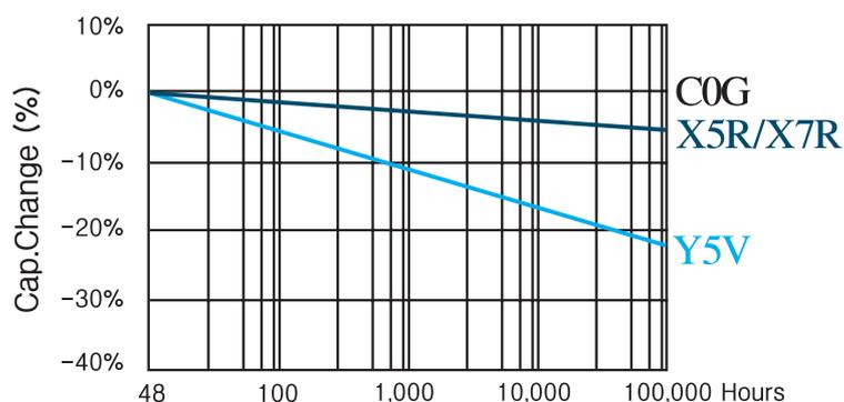
The capacitance value can be restored(also known as 'de-aged') by exposing the component to elevated temperatures approaching its curie temperature(approximately 120°C). This 'de-aging' can occur during the component's solder-assembly onto the PCB, during life or temperature cycle testing, or by baking at 150°C for about 1 hour.
