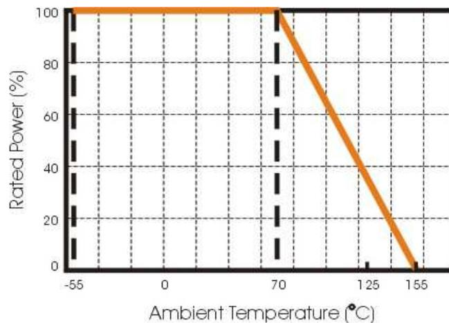
Figure 3. Maximum dissipation in percentage of rated power as a function of the ambient temperature.
