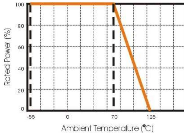
Figure 2. Maximum dissipation in percentage of rated power
