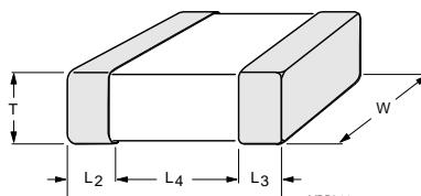
Fig. 2 Surface mounted multilayer ceramic c
