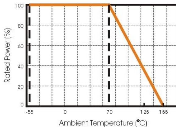
Fig.2 Maximum dissipation in percentage of rated power
