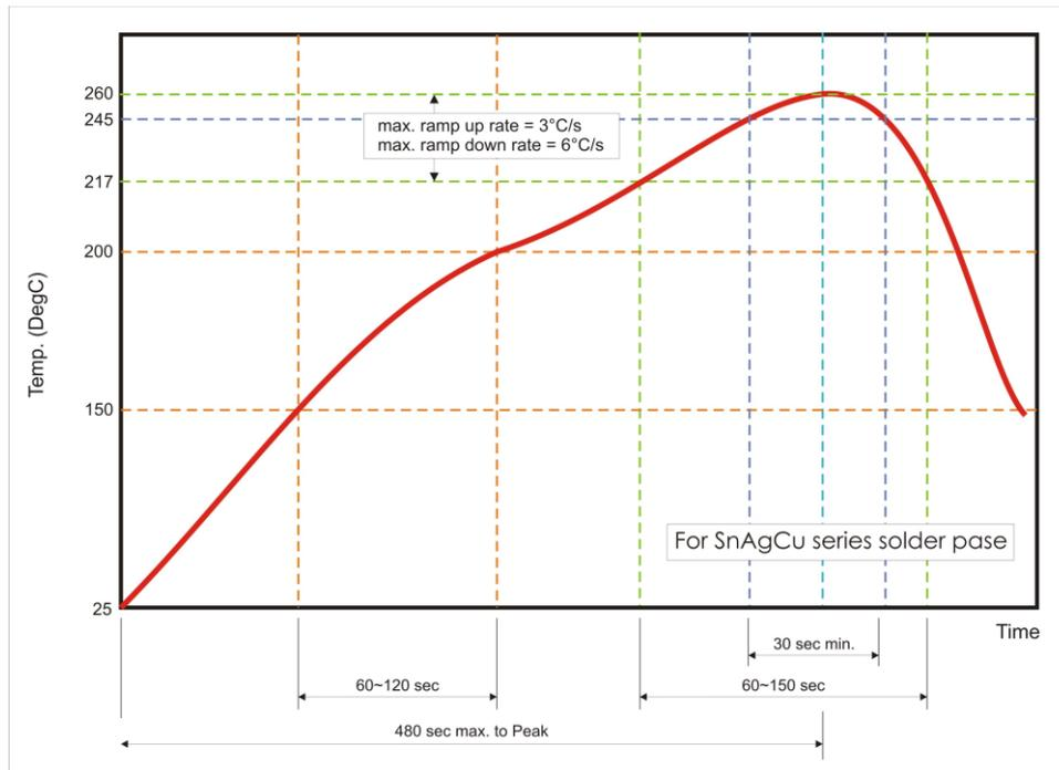
**Fig 3. Infrared soldering profile for Chip Resistors**
