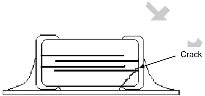
6. Handling of Loose Chip Capacitor
